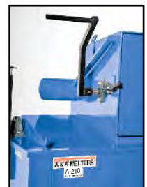
Lock safety tray open or closed with easy turning handle.
