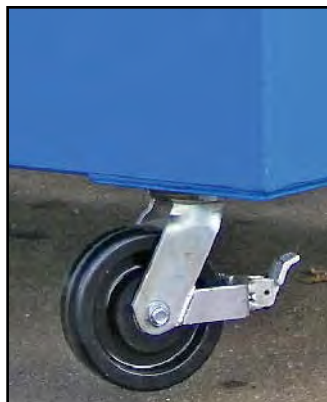
Optional 8" locking castor wheels, rated 2000 lbs each.
