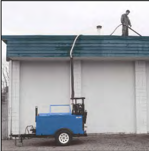
Boom stands upright or can be converted to a rigid pipe for greater heights
