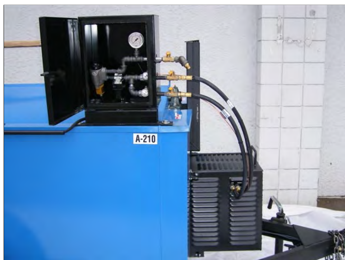
ATC System Designed for Ease of Use in the Field Comes in a Fully Self-contained Lockable Box.
