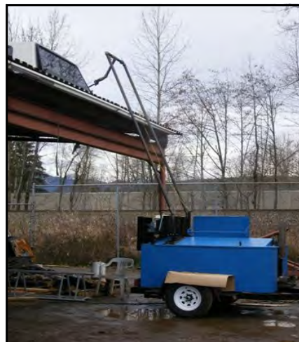
Recirculating system keeps the pipe hot to eliminate freeze up
