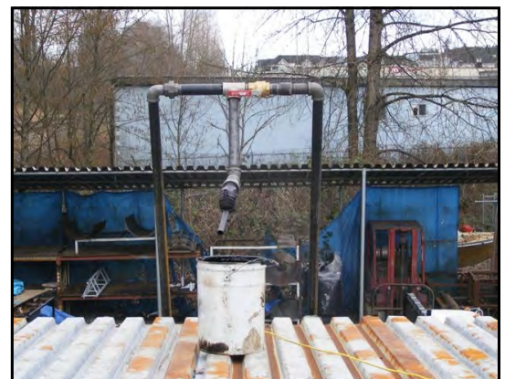
Recirculating system keeps the pipe hot to eliminate freeze up
